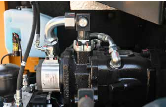
Load Sensing System The maximum flow rate of the main pump is 158.4+17.6lpm. New load sensing system provide faster independent action a low fuel consumption.
