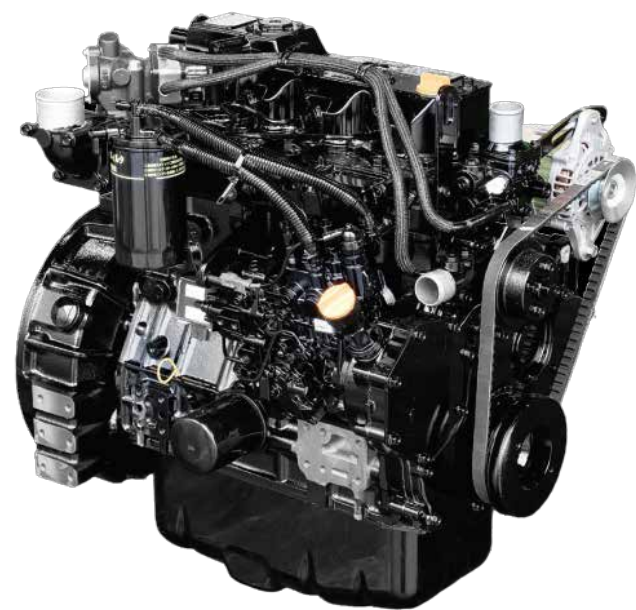
Yanmar Engine 4TNV98-Z Yanmar Engine, Output is 59.5HP/ 2,100 rpm, the maximum torque of 240.3N · m/ 1,575 rpm. ※ For best performance, engine should be operated at altitudes less than 1,200 m.
